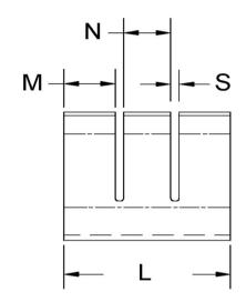
ALL DIMENSIONS ARE TO BE MEASURED WITH THE SPRING CLIP SECURED TO A FLAT SURFACE AND A COMPONENT OF THE NOMINAL DIAMETER IN PLACE.
