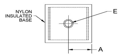
ALL DIMENSIONS ARE TO BE MEASURED WITH THE SPRING CLIP SECURED TO A FLAT SURFACE AND A COMPONENT OF THE NOMINAL DIAMETER IN PLACE.
