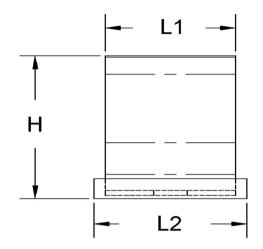
ALL DIMENSIONS ARE TO BE MEASURED WITH THE SPRING CLIP SECURED TO A FLAT SURFACE AND A COMPONENT OF THE NOMINAL DIAMETER IN PLACE.
