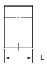
ALL DIMENSIONS ARE TO BE MEASURED WITH THE SPRING CLIP SECURED TO A FLAT SURFACE AND A COMPONENT OF THE NOMINAL DIAMETER IN PLACE.
