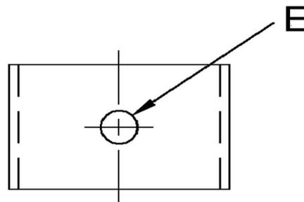
ALL DIMENSIONS ARE TO BE MEASURED WITH THE SPRING CLIP SECURED TO A FLAT SURFACE AND A COMPONENT OF THE NOMINAL DIAMETER IN PLACE.
