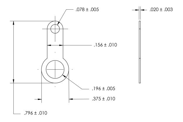
NOTES 1. SILVER PLATE PER ASTM B700 TYPE 1 GRADE A CLASS S, 2.5 $\mu$ m TH w/NICKEL UNDERPLATE
