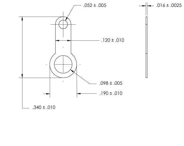
NOTES 1. TIN-LEAD DIP PER MIL-DTL-14072, M258. MUST CERT SOLDERABILITY TO MIL-STD-202, M208 - REFLOW ALLOWED, IF REQUIRED
