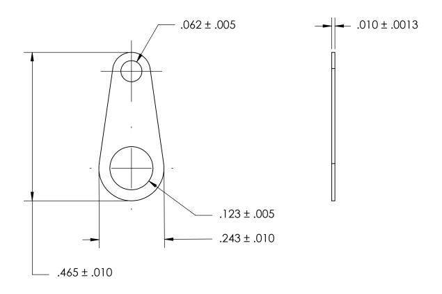
NOTES 1. SILVER PLATE PER ASTM B700 TYPE 1 GRADE A CLASS S, 2.5µm TH w/NICKEL UNDERPLATE
