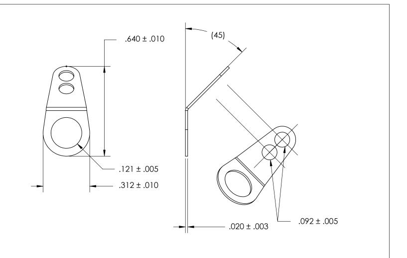
NOTES 1. SILVER PLATE PER ASTM B700 TYPE 1 GRADE A CLASS S, 2.5µm TH w/NICKEL UNDERPLATE
