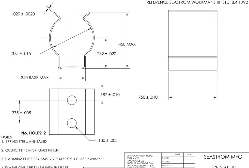
4. DIMENSIONS ARE TAKEN WITH THE PART CLAMPED TO A FLAT SURFACE AND A DUMMY COMPONENT IN PLACE.
