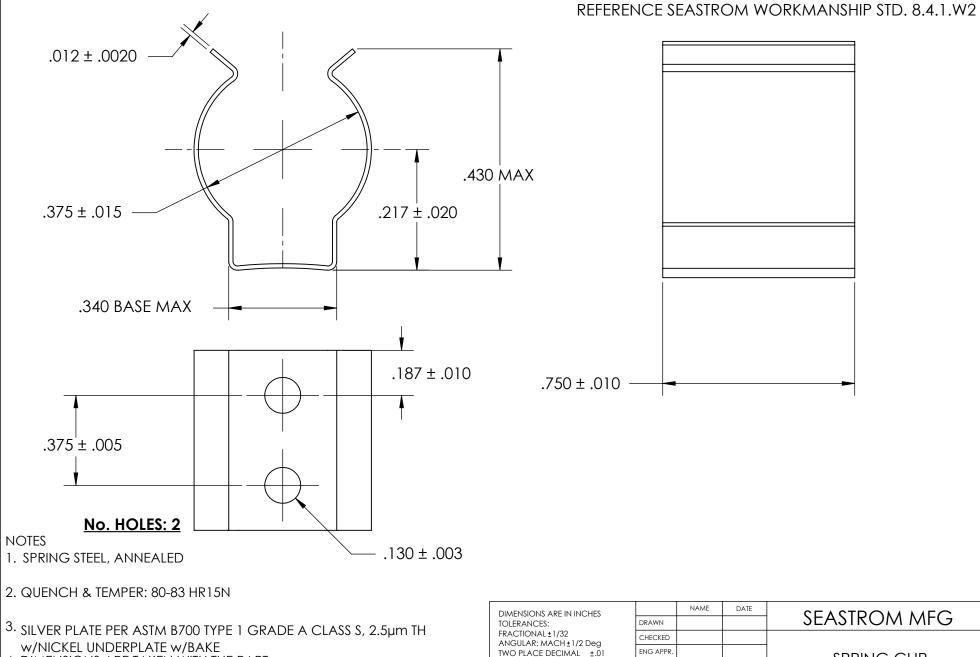
4. DÍMENSIONS ARE TAKEN WITH THE PART CLAMPED TO A FLAT SURFACE AND A DUMMY COMPONENT IN PLACE.
