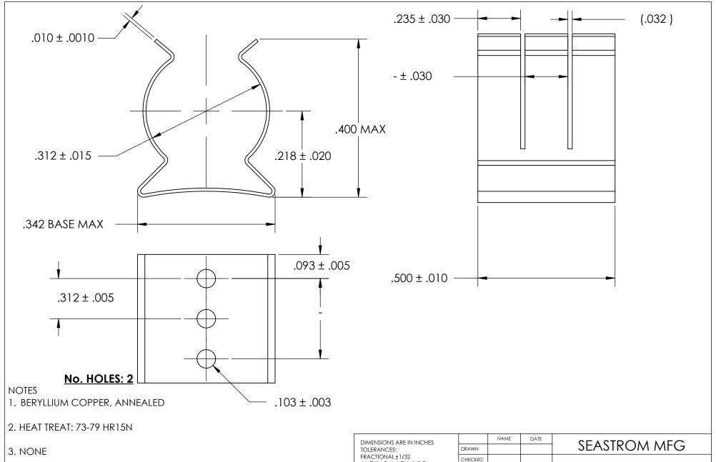
4. DIMENSIONS ARE TAKEN WITH THE PART CLAMPED TO A FLAT SURFACE AND A DUMMY COMPONENT IN PLACE.
