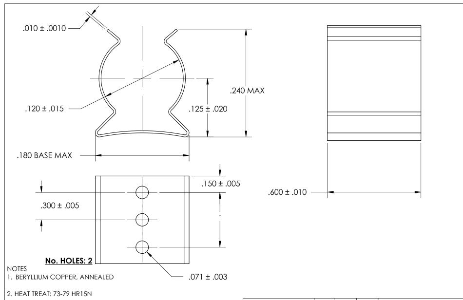
3. SILVER PLATE PER ASTM B700 TYPE 1 GRADE A CLASS S, 2.5µm TH W/NICKEL UNDERPLATE
