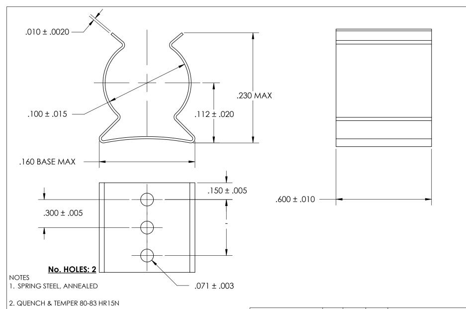
3. SILVER PLATE PER ASTM B700 TYPE 1 GRADE A CLASS S, 2.5µm TH W/NICKEL UNDERPLATE W/BAKE
