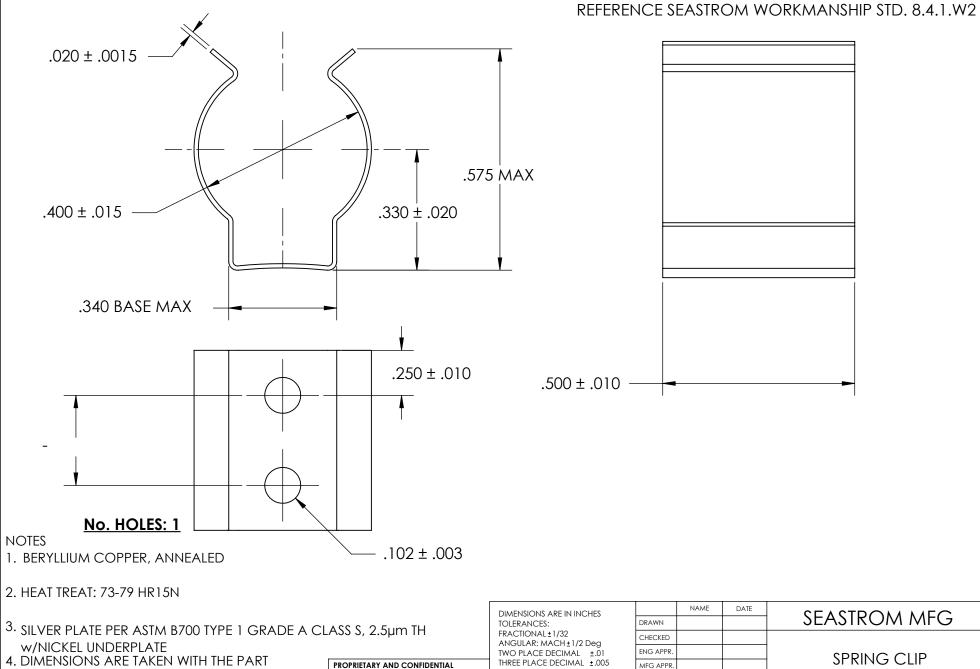
COMPONENT IN PLACE. 5. DIMENSIONS APPLY PRIOR TO PLATING.
