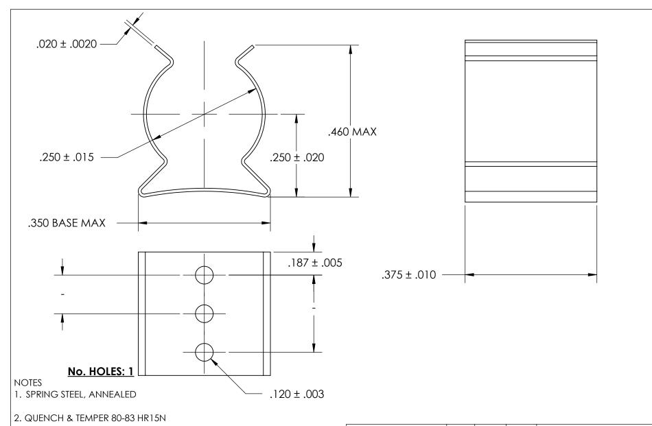
3. SILVER PLATE PER ASTM B700 TYPE 1 GRADE A CLASS S, 2.5µm TH W/NICKEL UNDERPLATE W/BAKE
