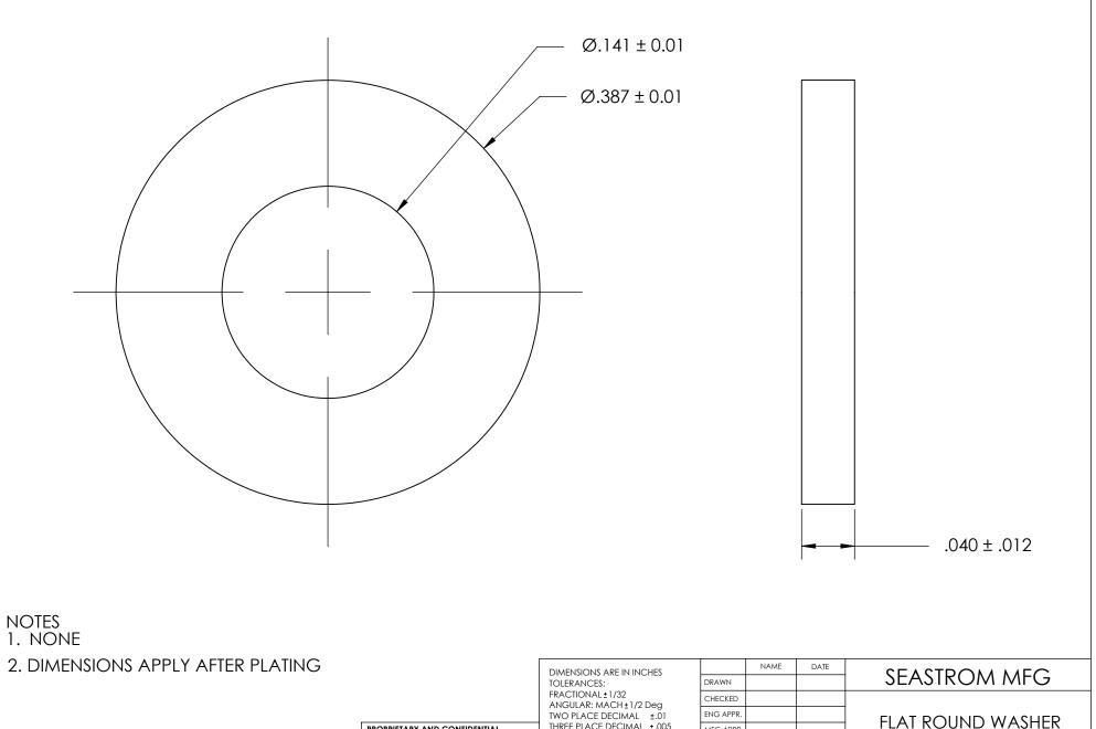
TWO PLACE DECIMAL ±.01 THREE PLACE DECIMAL ±.005 FLAT ROUND WASHER PROPRIETARY AND CONFIDENTIAL MFG APPR. THE INFORMATION CONTAINED IN THIS MATERIAL Q.A. DRAWING IS THE SOLE PROPERTY OF NEOPRENE COMMENTS: SEASTROM MANUFACTURING. ANY REPRODUCTION IN PART OR AS A WHOLE SIZE DWG. NO. 5613-3M-100 WITHOUT THE WRITTEN PERMISSION OF SEE NOTE 1 REV. SEASTROM MANUFACTURING IS PROHIBITED. DRAWING IS NOT TO SCALE SHEET 1 OF 1
