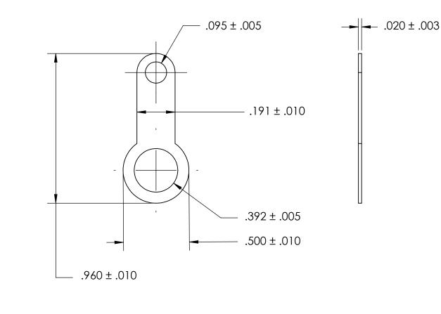
NOTES 1. TIN-LEAD DIP PER MIL-DTL-14072, M258. MUST CERT SOLDERABILITY TO MIL-STD-202, M208 - REFLOW ALLOWED, IF REQUIRED
