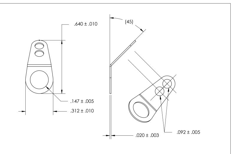
NOTES 1. SILVER PLATE PER ASTM B700 TYPE 1 GRADE A CLASS S, 2.5 $\mu$ m TH w/NICKEL UNDERPLATE
