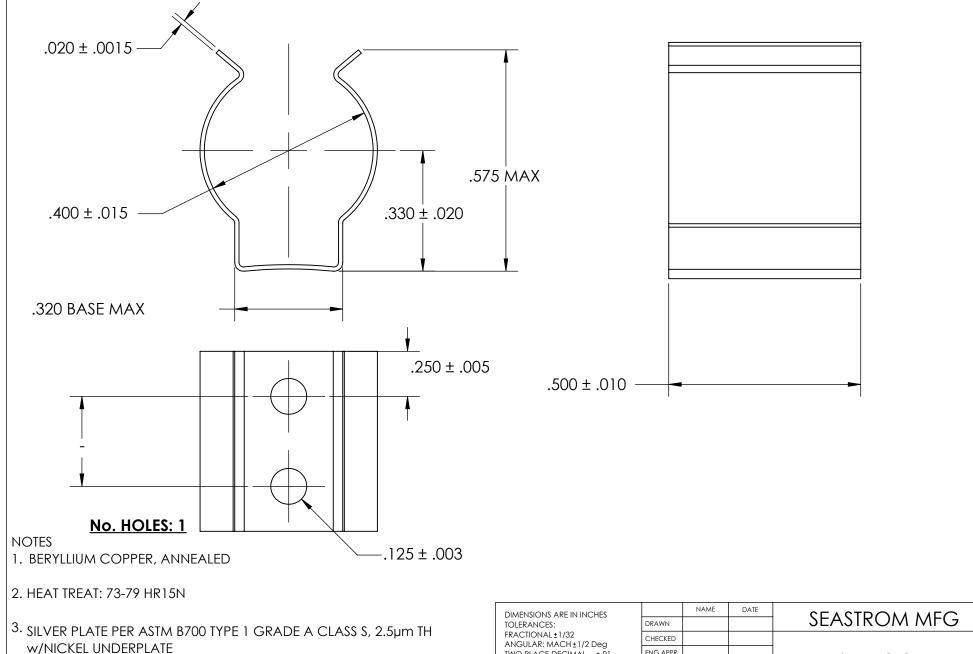
4. DÍMENSIONS ARE TAKEN WITH THE PART CLAMPED TO A FLAT SURFACE AND A DUMMY
