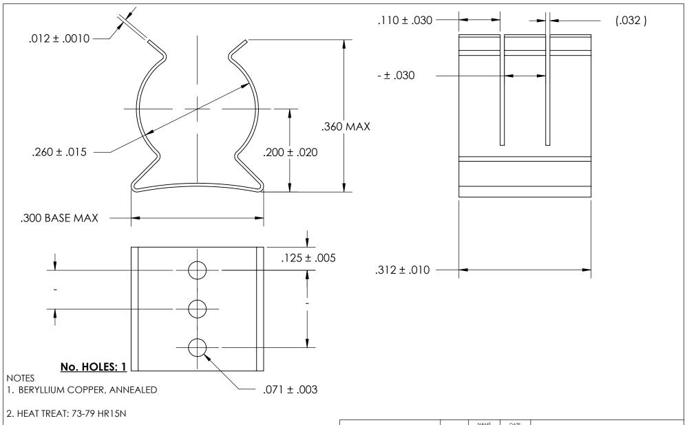
3. SILVER PLATE PER ASTM B700 TYPE 1 GRADE A CLASS S, 2.5µm TH W/NICKEL UNDERPLATE
