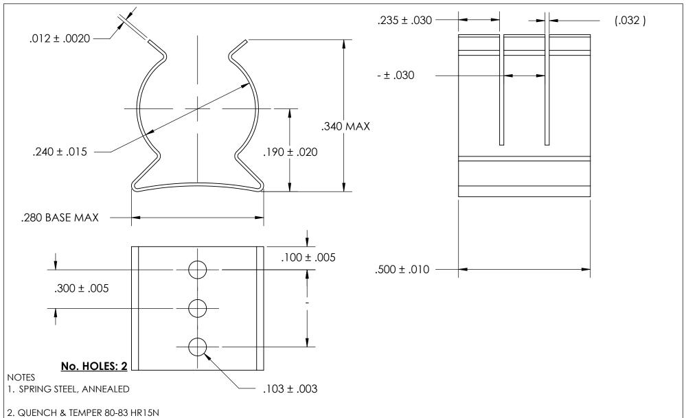
3. SILVER PLATE PER ASTM B700 TYPE 1 GRADE A CLASS S, 2.5µm TH W/NICKEL UNDERPLATE W/BAKE
