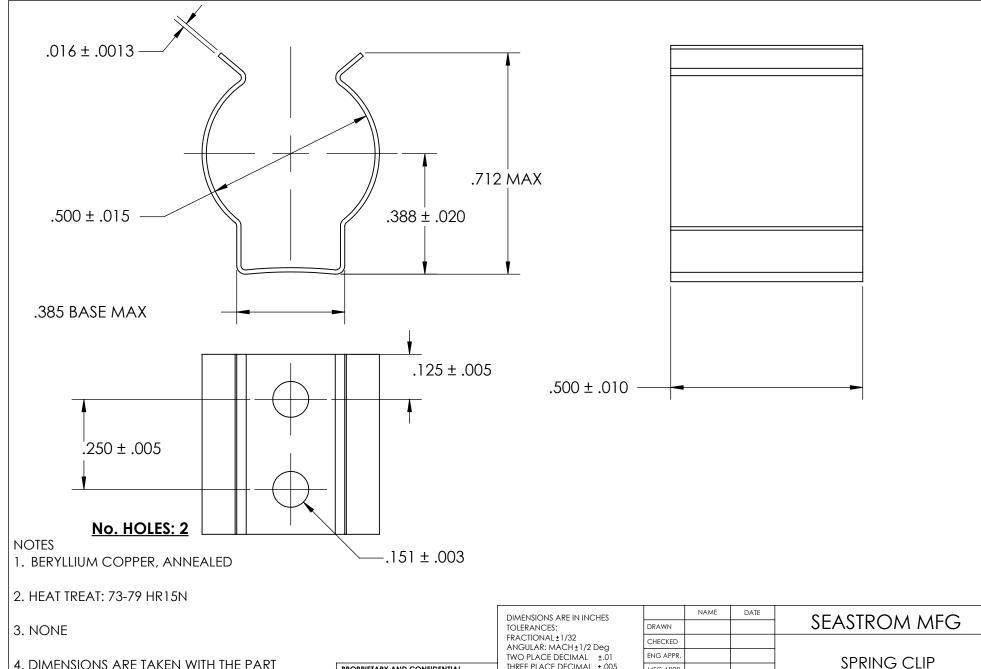
4. DIMENSIONS ARE TAKEN WITH THE PART CLAMPED TO A FLAT SURFACE AND A DUMMY
