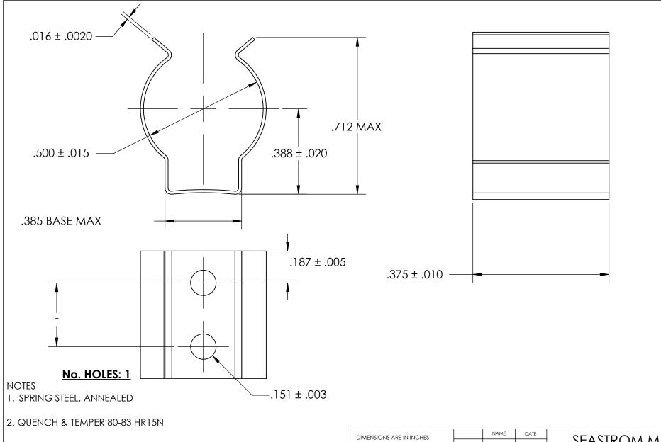
3. CADMIUM PLATE PER AMS QQ-P-416 TYPE II CLASS 2 w/BAKE
